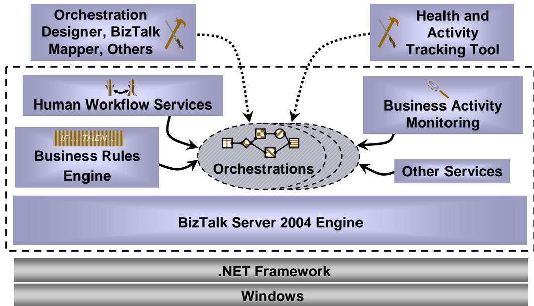
As the diagram indicates, BizTalk Server 2004 is built on the .NET Framework and runs on Windows. The core of the product, called the BizTalk Server Engine, is used by every orchestration. Other components may also be used depending on what's required for a particular application. The following sections describe these components and the engine that acts as the product's foundation.
