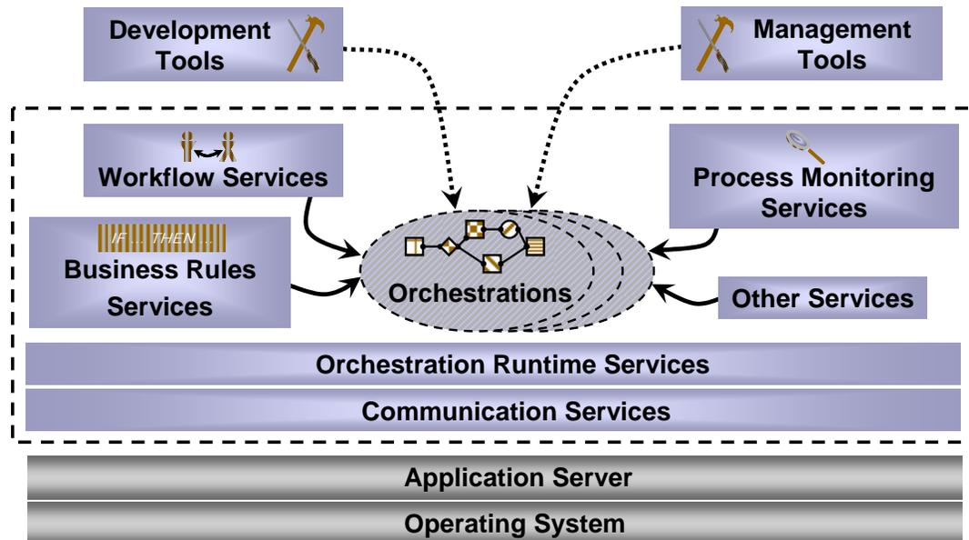
As the diagram shows, BPM server vendors commonly build their offerings on an application server, such as the .NET Framework or a J2EE-based product, which in turn runs on some operating system. On this foundation, a BPM server can provide a range of support for orchestrations, including the following:
